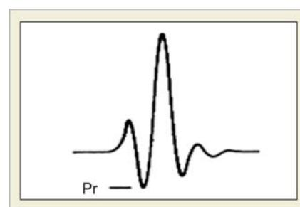
**Fig. 2:** Typical pulse wave of B-mode ultrasound: Mechanical index (MI) = Pr (mega-pascal)/ $\sqrt{\text{frequency (MHz)}}$ , Pr = rarefactional pressure (negative pressure), mechanical effect is caused by sound pressure, large mechanical effect of spectral Doppler is caused by long pulse, high pressure and high repeated frequency, MI should be 1 or less in obstetrics
