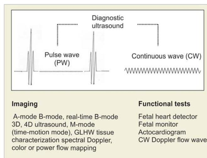
Fig. 1: Two types of ultrasound waves used in the diagnostic equipments
