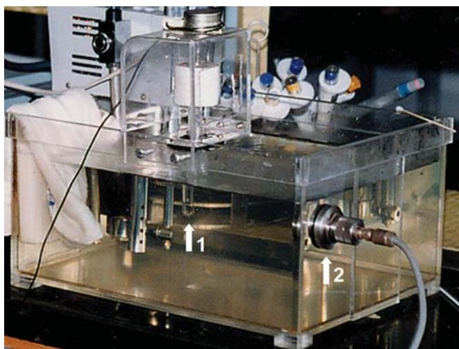
**Fig. 3:** Cultured cells were exposed experimental ultrasound in the 37°C water insulating the heat of transducer. The arrow 1 is cell container and arrow 2 ultrasound generating transducer. Pregnant animals were also exposed ultrasound in the water tank separating heated transducer, and no anomaly was produced in our group study
